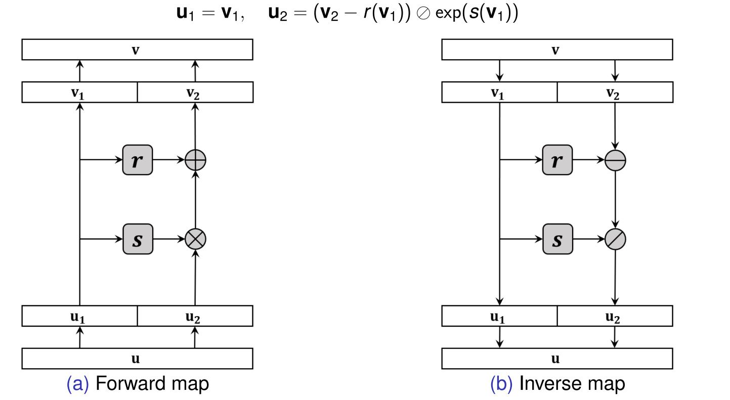
Figure: Coupling layer in normalizing flow.
