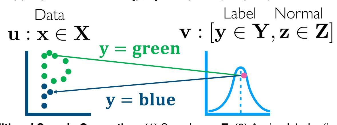
Figure: Conditional Sample Generation. (1) Sample  $z \sim Z$ , (2) Assign label y (i.e., color), (3) Inverse map to generate  $\mathbf{x} = f^{-1}([\mathbf{y}, \mathbf{z}])$  in the appropriate location.
